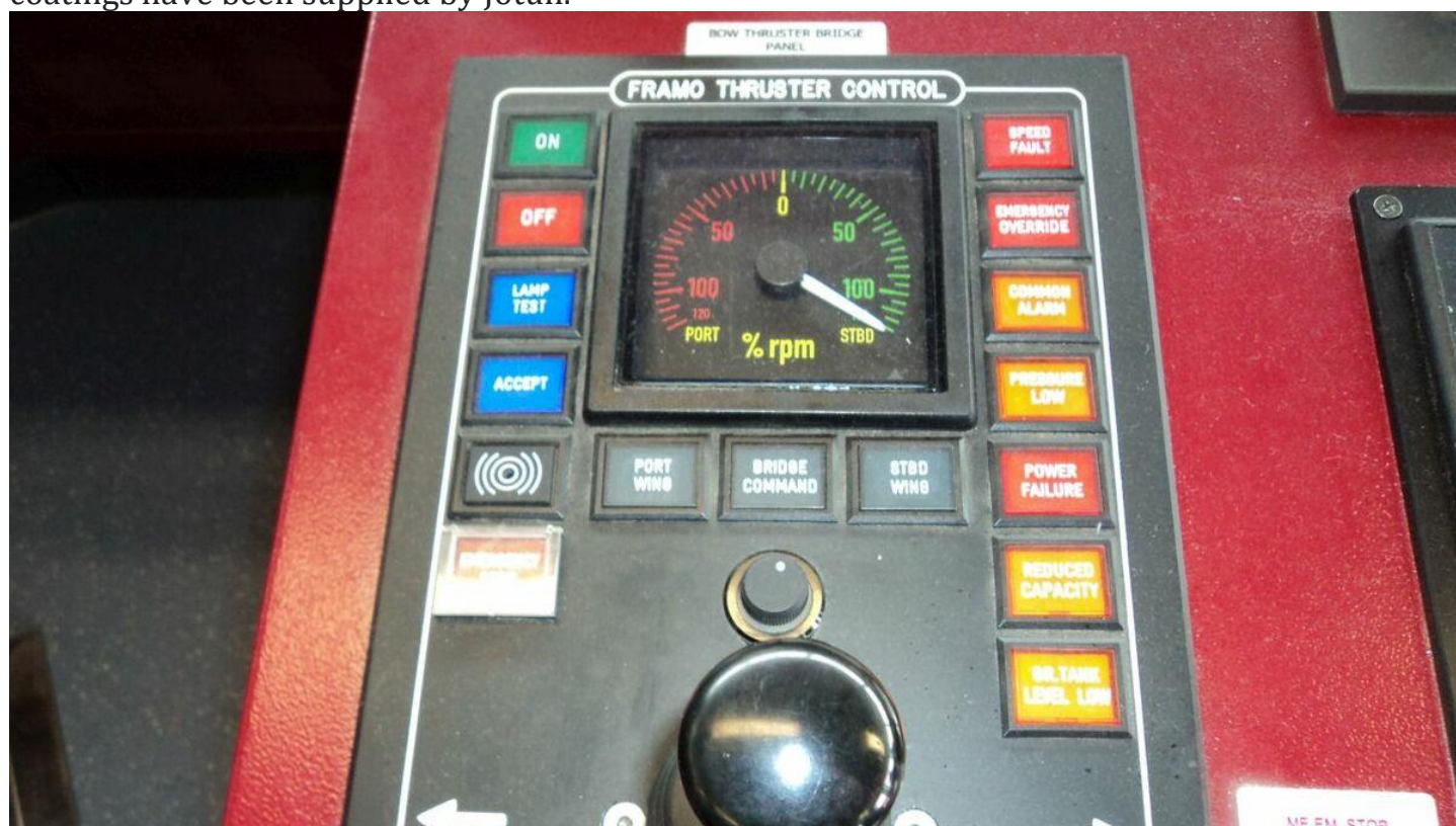
Framo is well known for pumps, but also supplied the thruster hydraulic controls
